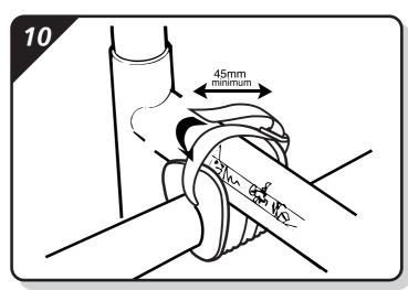
Position your cycle(s) into the saddle area of the frame locator. Pass the webbing strap over the frame of the cycle and thread through the metal loop. Pull the strap back tightly and press the hook and loop fastener to secure.
